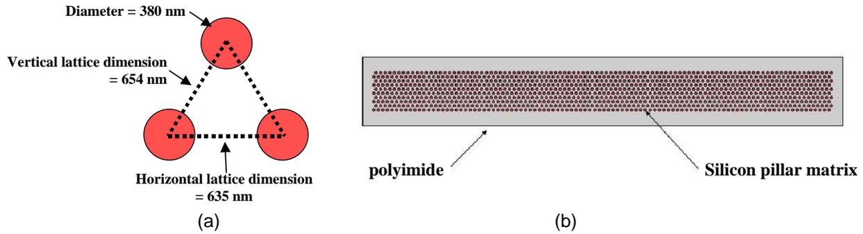
Figure 6. (a) Dimensions of the unit cell. (b) The entire photonic crystal structure layout which contains 10 rows with 100 pillars per each row.
