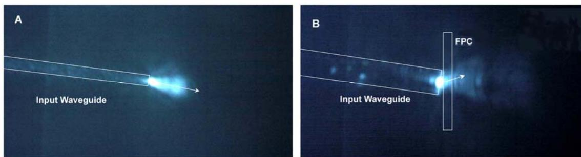
Figure 8. Collected light propagation images: (a) straight light propagation w/o PC; (b) giant negative refraction through the 2D slab Si/polymer PC.
