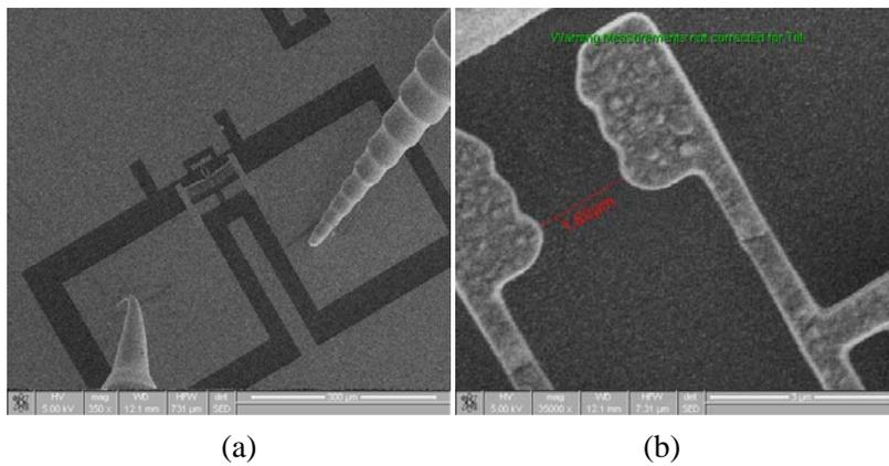
Figure 4. SEM images of: (a) the probes and the sub-micron gripper under test; (b) the gripper jaw opening (1.6  $\mu\text{m}$ ) with the applied current of 20 mA (4mW, 200 mV).
