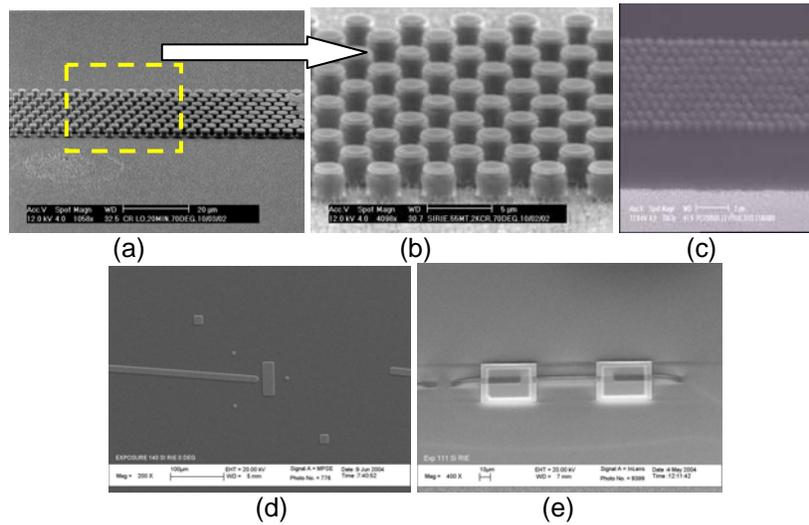
Figure 7. SEM photomicrographs: (a) anisotropically dry etched triangular array of circular silicon pillars with diameters in the range of 500 nm ~ 2.5  $\mu\text{m}$ ; (b) close-up view; (c) a triangular array of circular silicon pillar embedded in a patterned polyimide; (d) angled silicon waveguide; (e) air suspended FPC.
