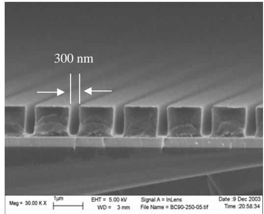
Figure 2. SEM image of high aspect ratio sub-micron electron beam lithography in PMMA.
