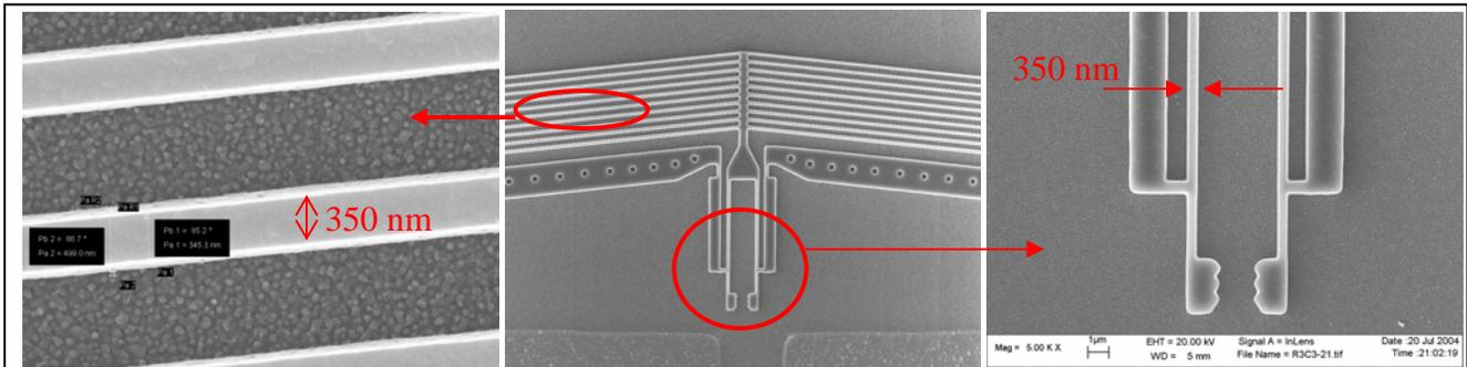
Figure 3. SEM images of a fabricated suspended submicron metallic electrothermal gripper with the bent-beam width of 350 nm, the gripper jaw opening of 2.1  $\mu\text{m}$ , and the structural thickness of 1  $\mu\text{m}$ .
