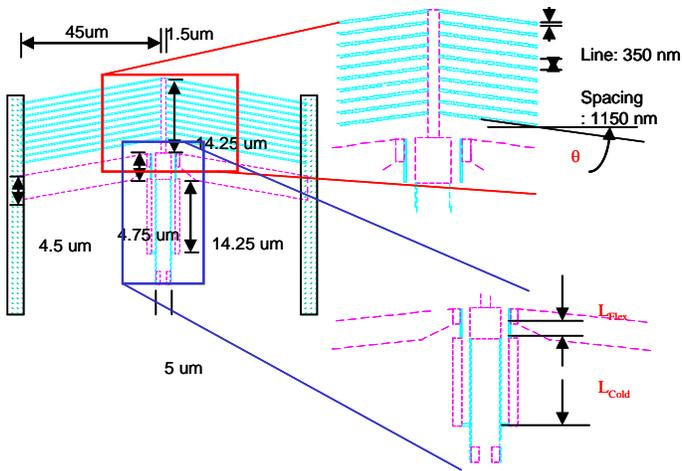
Figure 1. Schematic diagram of the sub-micron gripper design.
