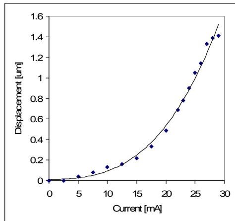
Figure 5. Amount of displacement of the sub-micron gripper as a function of the applied current.
